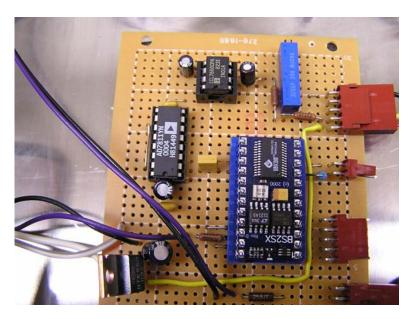
Figure 17. View of microprocessor and associated hardware for prototype hose conditioning device.
