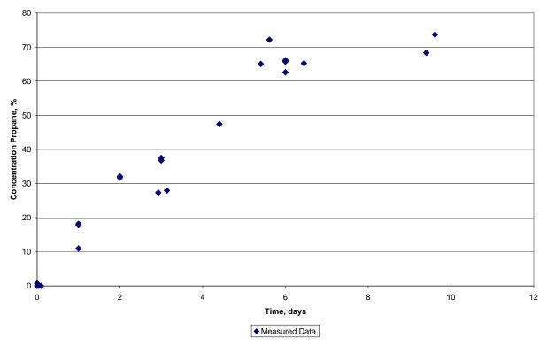
Figure 13. Plot of permeation data from dynamic rig testing on 1-inch diameter, 2-foot hose at 5 gpm and 150 to 200 psi.
