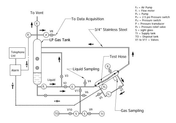
Figure 3. Schematic of test setup for periodic removal of LPG samples from test hose.
