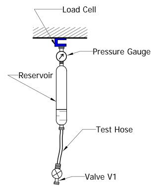
Figure 14. Test setup for load cell measurement.
