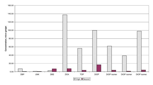
Figure 12. Extraction rates for virgin and second exposure in hose with 1/4-inch diameter.
