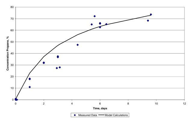
Figure 15. Measured propane permeability for samples taken with plastic and glass syringes and model calculation (solid line).
