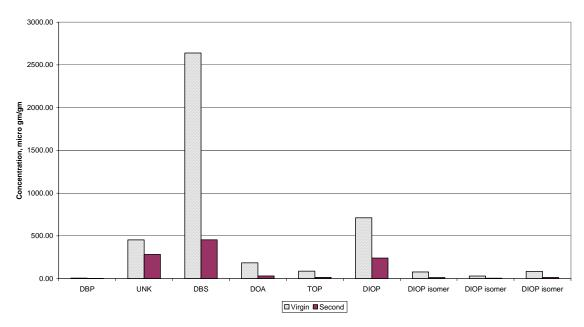
Figure 10. Extraction rates for virgin and second exposure in hose with 1-inch diameter.
